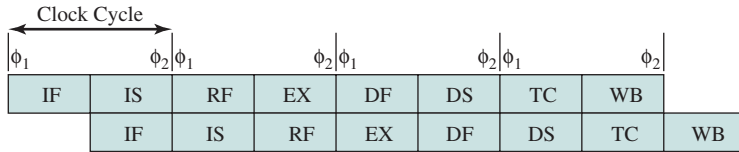
(b) R4000 pipeline
